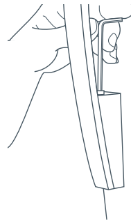
Fig.2c Tighten the handle screw with Allen key
